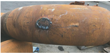
(c) 弯管上工装焊疤形貌
